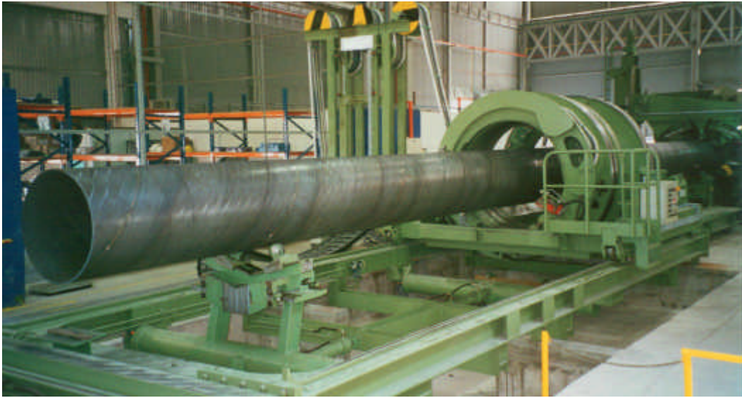
A part of the spiral pipe forming and tack-welding machine can be seen on the above photograph.
